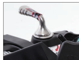
LARGER CLUTCH LEVER FOR EASE OF USE WITH GLOVES
