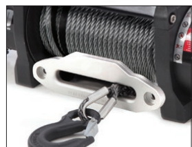
COMP SERIES ALUMINUM FAIRLEAD AND SYNTHETIC ROPE
