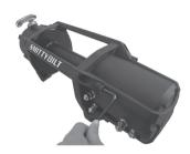
Step 1: Loosen and remove the 4 mator bracket bolts
