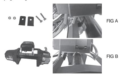
Step 2: Determine where you want control box over the drum (left, center, right), then secure using the included screw, L bracket, nut on the rear. The screw goes through the aluminum bracket and into the L bracket with the bottom of the L bracket placed into the slot of the rear tie-bar and finally secured more with included lock nut. (Fig A,B)
